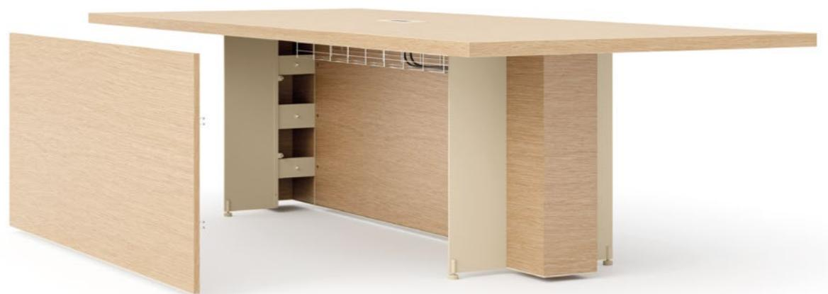
The two modesties are designed to allow easy and tidy cable management. One panel is fixed and structural, the other one is removable. The latter allows access to an horizontal metal basket used to run the cables.
